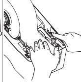
label width by turning the guide adjuster knob.
