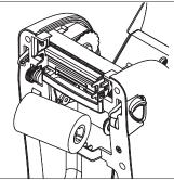
(3) Insert the ribbon right side onto the supply hub. Align the notches on the left side and mount onto the spokes.
