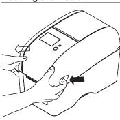
(1) Open the printer top cover by pulling the tabs located on each side towards the front of the printer, and then lift the top cover to the maximum open angle.
