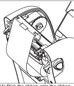
(4) Stick the ribbon onto the ribbon rewind paper core and insert the paper core onto the rewind hub.
