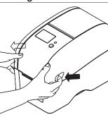
(1) Open the printer's top cover by pulling the top cover open levers located on each side of the printer and lifting the top cover to the maximum open angle.
