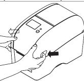
(1) Open the printer top cover by pulling (2) A top cover support at the rear of the tabs located on each side towards the front of the printer, then lift the top cover to the maximum open angle.
