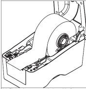
(4) Place the paper, printing side face up, (5) Move the media guides to fit the through the media guides, media sensor and place the label leading edge onto the platen roller.
