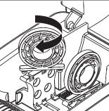
(2) The media holder can be used for 1" and 1.5" media core by rotating the upper part of label holder 180 degrees clockwise.
