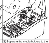
label roll width. Place the roll between the holders and close them onto the core.
