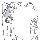
(5) Turn the ribbon rewind gear until the ribbon plastic leader is thoroughly wound and the black section of the ribbon covers the print head. Close the ribbon access cover and the top
