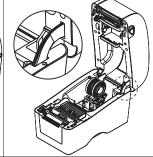
the printer will engage with lower inner cover to hold the printer top cover open.
