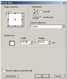
Now click on OK. The label is now shown as a grey frame on a white background. Everything inside of the blank area will be printed and after printing the LabelMax SP2 will cut off the tape (e.g. after 100mm as shown in the picture).
