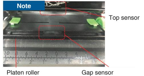
4. Feed the paper, printing side face up, through the media guides and place the label leading edge onto the platen roller. Move the media guides to fit the label width.
