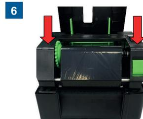
5. Close the print head mechanism with both hands and make sure the latches are engaged securely.
