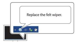
The felt wiper is a component used for cleaning the print heads. When the message shown in the i gure appears on the Utility icon on the computer task tray, it is time to replace the wiper with a new one. To purchase a felt wiper, contact us directly or your authorized MAX Systems Distributor.
