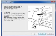
Manual Head Cleaning procedures are displayed. Carefully read the on-screen instructions and start the cleaning tasks.
