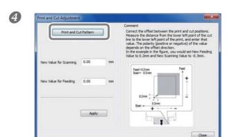
Click [Print and Cut Pattern]. The test pattern is printed.
