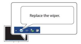
The wiper is a component used for cleaning the print heads. When the message shown in the i gure appears on the Utility icon on the computer task tray, it is time to replace the wiper with a new one.
