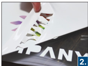
Weed (remove excess material).
