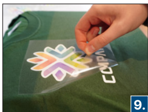
Remove the transfer film from the textile before it cools down (hot peel).
