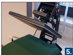
Preheat the heat press / iron (low temperature: 120 °C / quick application: 140 °C).
