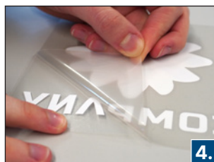
Carefully remove the carrier material from the textile film. The printed design must now adhere to the transfer film.
