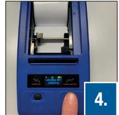
Open the label cover (1) on the top of the LabelMax MP1 and insert the foil tape (2) into the device. Slide the side guide up to the foil tape to ensure a straight run of the material. Please make sure that the (foil) side to be printed is at the bottom. (3). Now push the foil in the guides against the feed roll until you notice a resistance. Next, press the „Feed“ key to feed the material (4).
