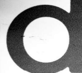
Dragging occurs when dirt around the print heads comes into contact with media.
