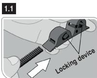
Insert band into closed side of the buckle.
