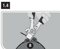
Use tightening tool to tighten band.
