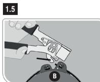
Use cutter blade on tool to remove excess band.
