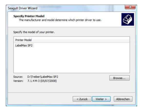
**Note**: The printer name should not be renamed. If this can not be avoided, the printer has to be renamed in the cadlink.ini as well (C:\SignMax\SignMax).
