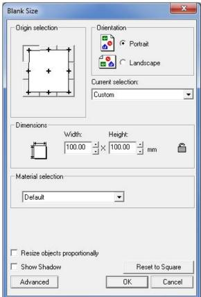
Set the label dimensions via "Layout", "Blank Size..." by entering its width and height in mm. Now click on OK. The label is now shown as a grey frame on a white background. Everything inside of the blank area will be printed and after printing the LabelMax SP2 will cut off the tape (e.g. after 100mm as shown in the picture).
