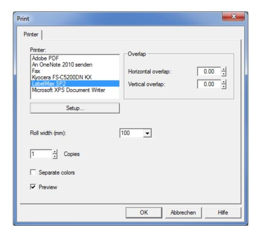
Very important is the field "Roll width". Here it is essential to select the correct roll width of the tape which is used in the printer right now.
