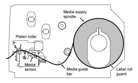
(7) Using the front display panel, set media sensor type and calibrate the selected sensor (See "Media Sensor Calibration" on facing page).
