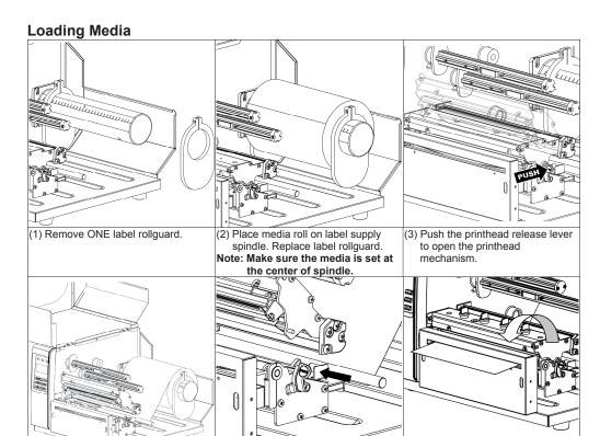
(4) Pull the leading edge of the label forward through the media guide bar past media sensor, and place the leading edge onto the platen roller. (5) Adjust the label guide to fit label width.
