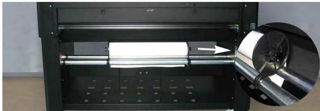
5. Press the bottom pushbutton (1), located on the right side, to unwind the media roll. Hold the media so it does not touch the floor. Insert the vinyl between the cassette station and the base. Make sure it is loaded far enough so that the beginning of the vinyl is underneath the clamp. Press pushbutton again.
