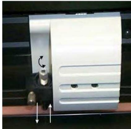
6. Close the clamp and tighten the clamp screw.
