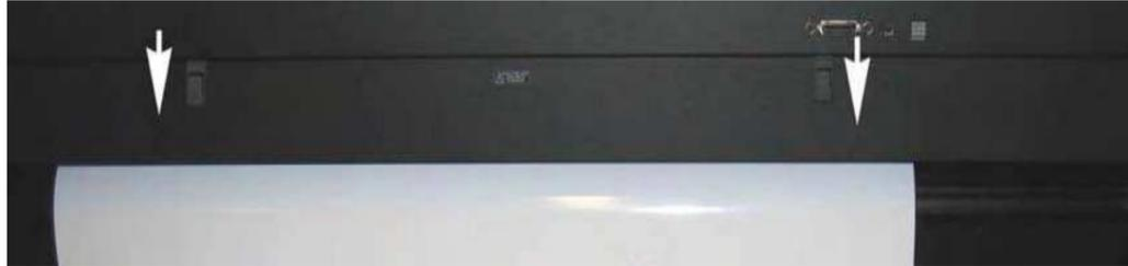
To remove a cassette, lift it enough to pass over the rubber bumper, then pull it backwards and out of the printer. To load a cassette, push it gently into an open location, until it just passes the rear bumper, then press it down and pull it backwards against the bumper.
