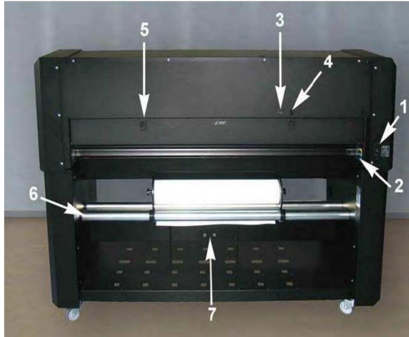
1. **Power Entry Module:** The fuse box, the AC power cord receptacle and the on/off switch are located in the power entry module. See section 1.4.3. for power up procedure and section 1.4.3. for information about changing the fuse.
