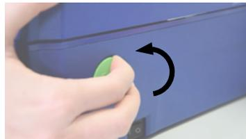
1. Open LabelMax SP3's top cover by pulling the top cover open levers and lifting the top cover to the maximum open angle.
