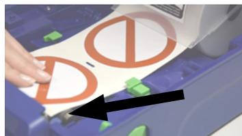
3. Remove the „LabelMax SP3 sealing“, pull of the Vinyl-tape and lay it down on the platten roller.
