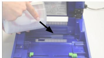
2. Watch the lands of the vinyl cartridge, they have to line up exactly with the notches in the LabelMax SP3.
