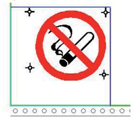
The registration marks are plotted for each color, so that you can use them when applying the foils. Use the mouse to move the registration marks. Click the sort Cut Order by Color" button in the Cut Toolbox. The "Sort Cut Order by Color" window opens.
