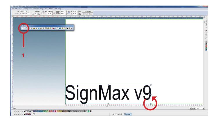
Use Button 1 to rotate the object and make optimal use of the foil. Afterwards, click the scissors in the Cut Toolbox. The cut job starts.
