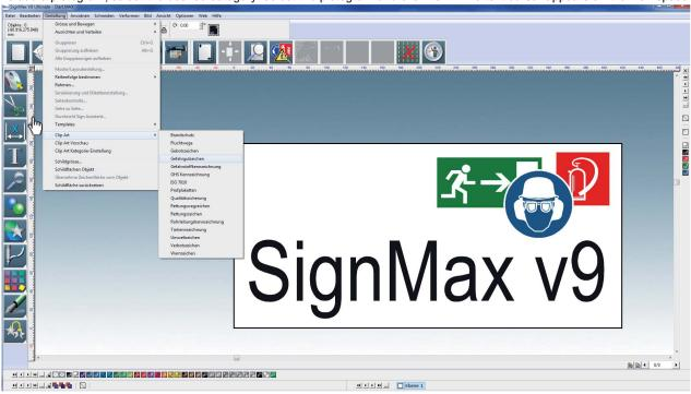
move the cursor to the correct position and click the left mouse button. The pictogram has its original size when inserted. If you keep the left mouse button pressed and drag a frame, you can specify the size when inserting the pictogram. Note: If there are no objects on the sign plate, the sign plate is automatically adapted to the pictogram.
